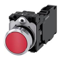
Pushbutton, 22 mm, round, metal, shiny, red, pushbutton, flat, momentary contact type, with holder, 1 NO+1 NC, screw terminal, with laser labeling, upper case and lower case, always upper case at beginning of line
