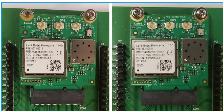
Figure 6: Attaching a 453-00011 Pinnacle™ 100 modem to a DVK
