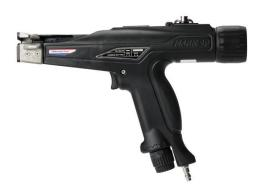
MK9 Pneumatic - Handle Air Supply Connection, includes tool and quick connect fittings.
