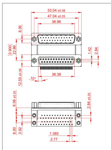
**ISSUE NUMBER** THIS IS A C.A.D. GENERATED DRAWING TOLERANCE UNLESS OTHERWISE SPECIFIED ORIGINAL (1)DO NOT MAKE MANUAL REVISIONS TO MASTER. .X ±0.25 .XX ±0.13 .XXX ±0.10 6.0 **3.18** ±0.38 6 İΤ TU 5.8 19.6 NOTES: MATERIAL: HOUSING: THERMOPLASTIC POLYESTER, UL94V-0, **BLACK IN COLOUR** SHELL: STEEL, NICKEL PLATED CONTACT: COPPER ALLOY, 15µ GOLD PLATING OPERATING TEMPERATURE: -55°C ~ 85°C **3A PER CONTACT**
