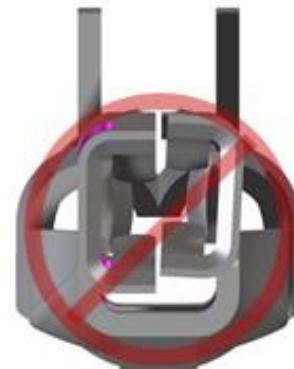
Damaged Front Box
