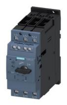
Circuit breaker size S2 for motor protection, Class 20 A-release 18...25 A N-release 325 A Screw terminal Standard switching capacity with transverse auxiliary switches 1 NO+1 NC
