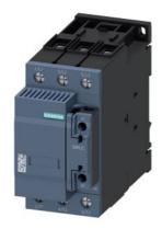
Capacitor contactor, AC-6b 50 kVAr, / 400 V 2 NC, 230 V AC, 50 Hz 3-pole, Size S2 screw terminal
