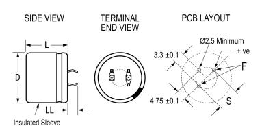
**General Information** Series PEH526 Dielectric Aluminum Electrolytic Description Snap-In, Aluminum Electrolytic RoHS Lead 3 Pin Short AEC-Q200 Qualifications AEC-Q200 Yes Component Weight 12 g Notes Add 0.5mm To D And 1mm To L For Sleeving. Shelf Life 520 Weeks
