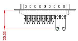
POWER/CO-AX CONTACT RATING:40A (CURRENT)(IF PRESENT)SIGNAL CONTACT CURRENT RATING:5A PER CONTACTSIGNAL CONTACT RESISTANCE: $10m\Omega$  MAX.INSULATOR RESISTANCE:5000MΩ min.DIELECTRICDIELECTRIC
