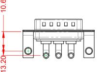
30A (CURRENT) **POWER/CO-AX CONTACT RATING:** (IF PRESENT) SIGNAL CONTACT CURRENT RATING: 5A PER CONTACT SIGNAL CONTACT RESISTANCE:  $10m\Omega$  MAX.
