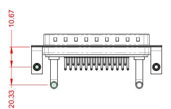
POWER/CO-AX CONTACT RATING:40A (CURRENT)(IF PRESENT)SIGNAL CONTACT CURRENT RATING:5A PER CONTACTSIGNAL CONTACT RESISTANCE:10mΩ MAX.INSULATOR RESISTANCE:5000MΩ min.
