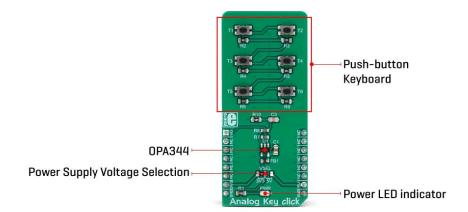
By pressing a button, the respective connection point becomes redirected to the input of the OPA344, a low-power operational amplifier from Texas Instruments, which is configured to work with the unity gain, forming a buffer for the input of the microcontroller (MCU). This prevents changes of the impedance at the MCU input pin, as well as a limited amount of ESD protection.
