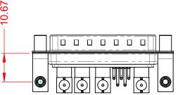
50Ω (IMPEDANCE) **POWER/CO-AX CONTACT RATING:** (IF PRESENT) SIGNAL CONTACT CURRENT RATING: 5A PER CONTACT SIGNAL CONTACT RESISTANCE:  $10m\Omega$  MAX. **INSULATOR RESISTANCE:**
